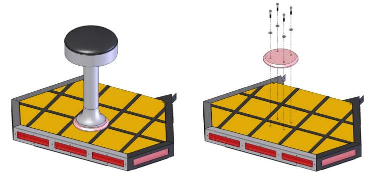
Remove the anti-slip tape from the platform to expose the fourteen screws that attach the floor to the stage. Now remove the floor. You can now access the fluorescent bulbs.
