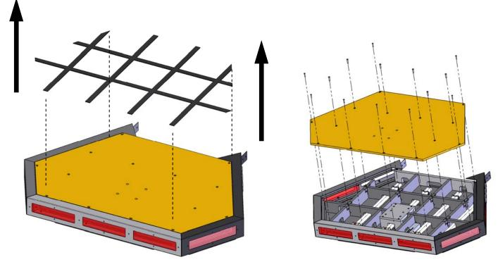
To replace bulbs 2,3, and 4 press the red button, remove the plastic retainers, lift up, and slide out as shown below. To replace bulbs 1 and 5 press the red button, remove the plastic retainers, and lift up and out as shown below.
