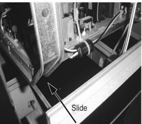
4. Connect 2 connectors from the upper cabint side to the monitor and 1 connector from the fan in the monitor box to the connector from the upper cabinet side.
