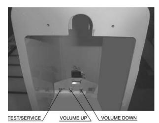
SERVICE/TEST BUTTON:To press this button gives credits without resistering the coin meter.<br/>Hold down this button to go into the TEST mode and press it in the<br/>TEST mode to select.VOLUME UP:Hold down this button in the attract mode to increase the sound volume.<br/>Press this button in the TEST mode to move cursor up.
