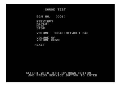
The advertize sound level can be adjusted by pressing VOLUME UP BUTTON and VOLUME DOWN
