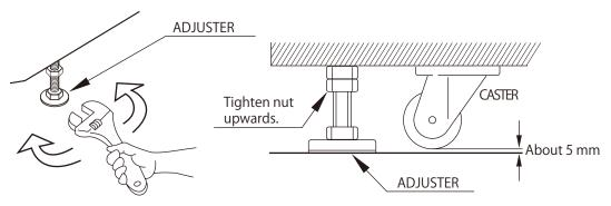
FIG. 6-11c Adjust the adjusters
