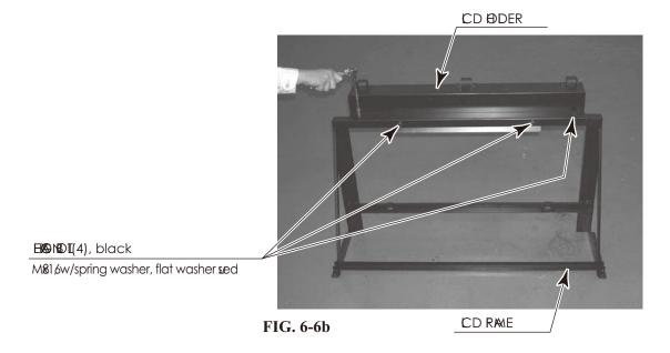
Place the LCD frame on the LCD base, and fix it with four hexagon bolts. The LCD frame and LCD base use flat washers with bolts that have spring washers attached.
