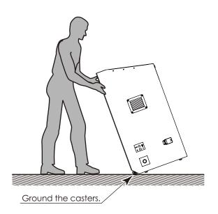
FIG. 7d Moving the control tower
