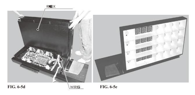
Fasten the ranking box by its bottommost frame to the ranking base with a total of eight screws. When fastening the screws, use either a short screwdriver or a ratchet handle with screwdriver tip. Each screw has a flat washer and spring washer attached.
