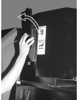
Replace the lamp. Be careful not to touch the glass surface of the front of the lamp. It is possible that it will burn out if oils from fingers are present.
