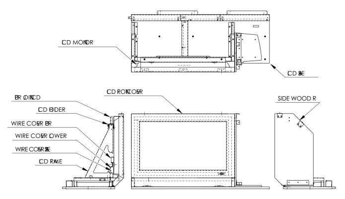
FIG. 6-6a LCD MONITOR
