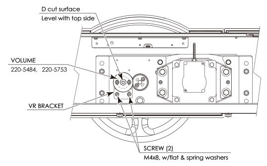
FIG. 10-1e STEERING WHEEL MECHANISM VOLUME
