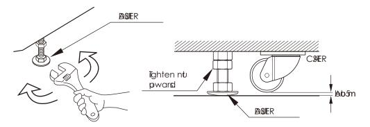
FIG. 6-4e Adjustment of adjusters
