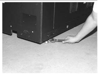
FIG. 6-4c Ground adjusters
