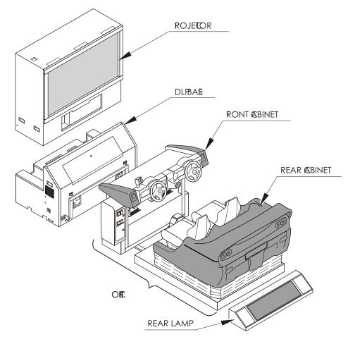
FIG. 6a Component parts of cabinet
