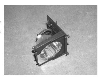
Remove the DLP front door. Remove the two truss screws that fasten the door.
