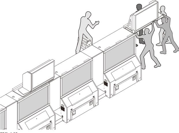
Move the LCD monitor to the fixing position. Align the left edge of the LCD monitor with the centerline of the four DLP projectors. Take care not to catch your hands or fingers.
