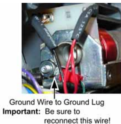
Figure 8. Gun Coil Assembly Service
