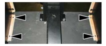
2. Next lower the Boom Mounted Display and place the Marquee so it goes over the Boom itself, and install the Marquee using 4x Philips screws provided shown by the arrows in the picture below.
