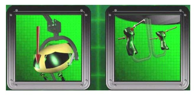
The Player Control Test will validate that the controls are setup correctly and working on the cabinet. When you press a button a red arrow will appear on the test screen when it is operating correctly as shown in the picture above. When you move the Headset in any direction a red arrow will appear in the direction that the Headset is moving when it is operating correctly. When you are finished testing the player controls press the Operator Button to exit back to the main operators menu.
