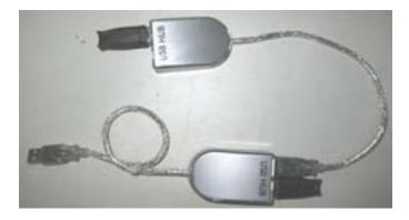
In the event that 2 USB HUB's are needed to create enough USB ports for all the game dongles you can daisy chain the USB HUBs together as shown above. Do not plug the USB cable coming from the HAPP GCI Controller card in the USB HUB's as this will cause the card to not work.
