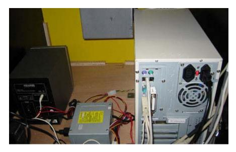
Connect the wall cord to a grounded (3-terminal) AC wall outlet.
