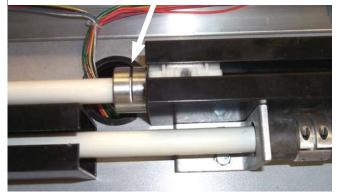
collar make sure the rod and gear box coupler touch, and retighten the gearbox. Be sure to leave 1/32" to 1/16" between the collar and the gearbox body.
